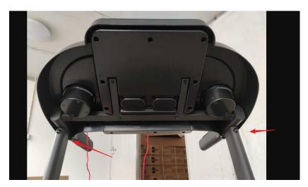
**Step 1:** locate the screws underneath the control plate. Unscrew these screws.
