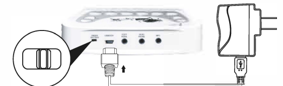
Battery Power Switch
