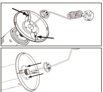
**4.** Secure the main body and base by turning the adjusting plastic screw nut clockwise.
