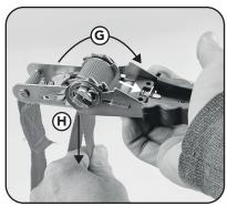
Ensure the ratchet fastener is in the flat position by pressing the release tab and overriding the ratchet end point (G). Pull on the non-fixed side of the webbing strap which will release the strap from the ratchet's hold. You'll then be able to completely pull and remove the strap through the bottom opening of the take-up spindle (H). Use the release tab to close the ratchet.
