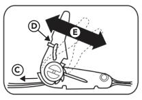
Once the excess slack has been pulled through (C), lift up the ratchet fastener (D) and simply move the fastener up and down (E) until the strap's tension is suitably tight. Finally close the fastener down to lock the ratchet in place. Ensure excess loose strapping will not tangle in truck/trailer wheels or interfere with moving parts.
