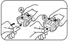
With the ratchet closed, feed one end of the strap through the take-up spindle (A) from the bottom upwards. Pull through the strap upwards from the take-up spindle and continue pulling all of the remaining slack in the direction shown (B).
