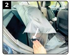
Pull the top edge of the seat cover down over the headrests. Pull the tether strap on one corner so that it attaches to a secure point on the rear of the bench seat. This will ensure that the seat cover won't come off.
