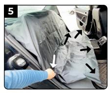
To finish off, ensure all edges of the seat protector covering the base of the bench seat are pulled as taut as possible for a snug fit.
