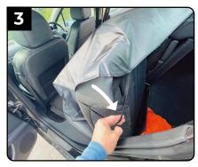
Repeat the process from step 2 with the other tether strap so that it's securely attached to a part of the seat's framework towards the rear.
