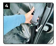
Start repositioning the seat belts from either side so that they are both not hidden and facing towards you. Then move the bench seat back to it's default fixed position ensuring the seat cover hasn't moved.
