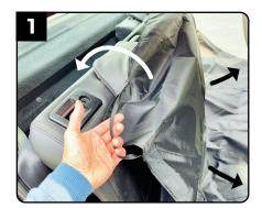
Adjust the headrests all the way down. Lower the bench seat by pressing the release latch and pulling the seat slightly forward. Drape the seat cover from the headrests down so it covers as much of the bench seat.
