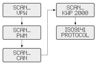
If a "LINK ERROR!" message shows up, turn the ignition off for about 10 seconds, check if the Scan Tool's OBDII connector is securely connected to the vehicle's DLC, and then turn the ignition back to on. Repeat the procedure from step 5. If the "LINK ERROR" message does not go away, then there may be problems for the Scan Tool to communicate with the vehicle.
