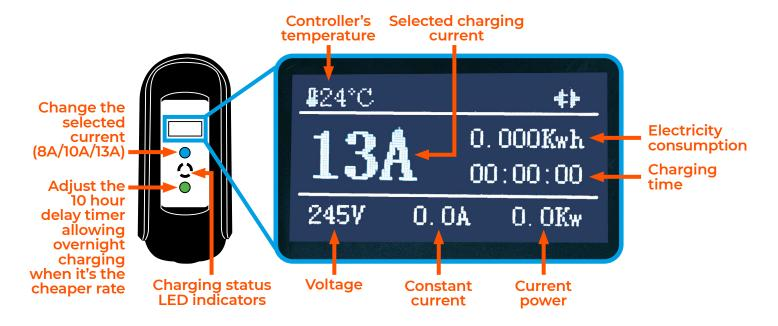
In order to switch charging current, make sure the power plug is firmly inserted into the mains socket and the charging plug end to the EV vehicle is disconnected, and then press the blue switch button (shown above). You will then be able to successfully adjust and set the charging current.
